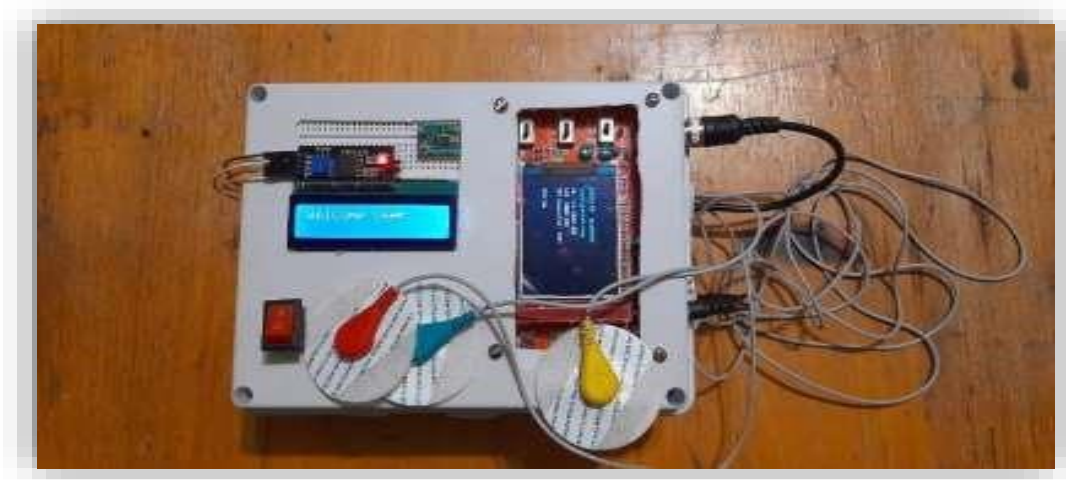
Figure 7: Integration of the ECG and pulse oximeter systems
