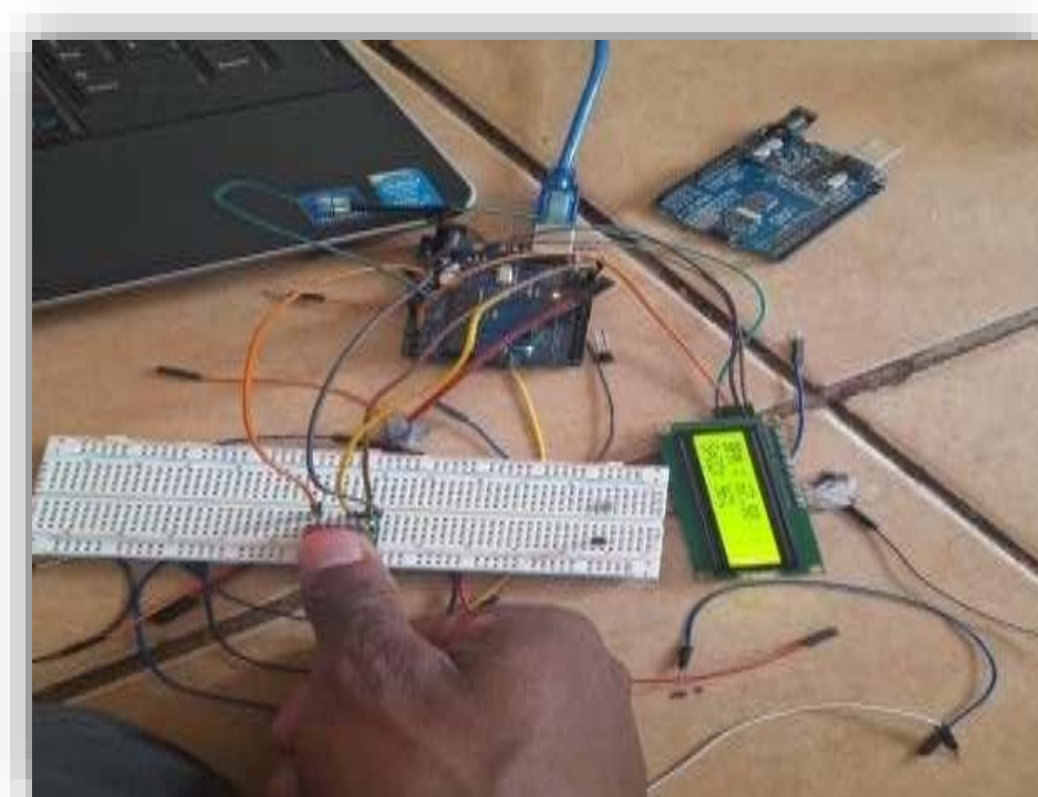
Figure 6: Fabrication of the pulse oximeter system
